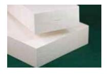
KLEERfold™ is a single piece of Kleer that is folded and laminated to produce a board with three finished sides. It is not for use in milling applications. KleerFold is available in the following nominal and (actual) sizes: 2" (1-1/2") x 4" (3-1/2") x 18' or 2" (1-1/2") x 6" (5-1/2") x 18'.
